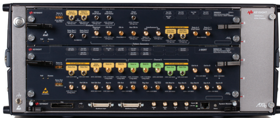
The M8062A multiplexer in a 32 Gb/s BERT setup with J-BERT M8020A
