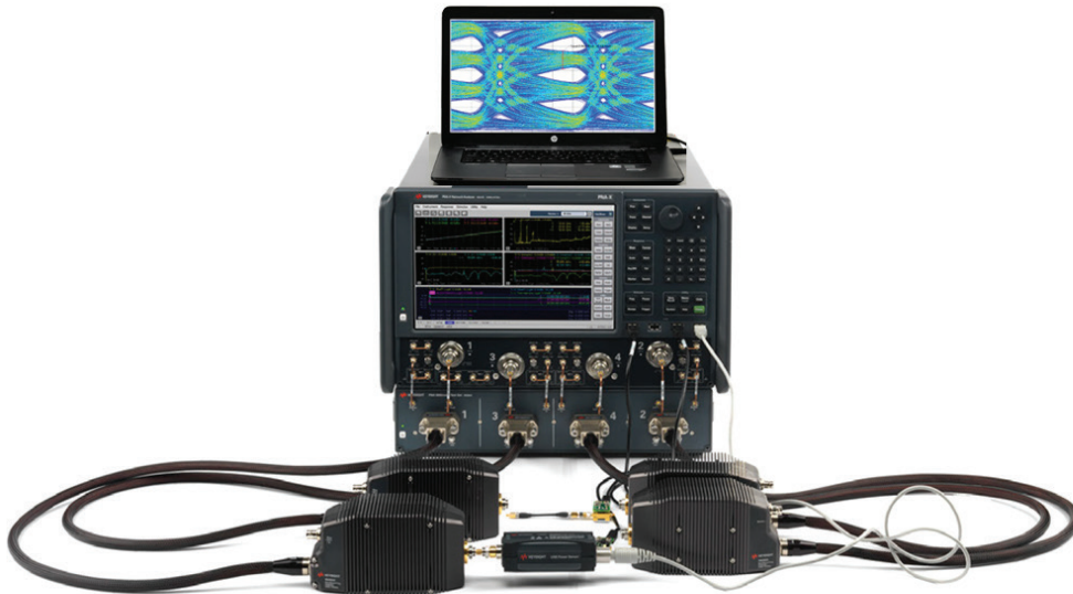
The N5291A enables PLTS 2018 to achieve 6-picosecond equivalent system risetime measurements providing better than 400-micron spatial resolution.
